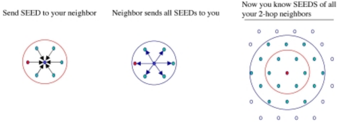
Figure 6: The fan-out and fan-in procedure for exchange seeds in a two-hop neighborhood.
